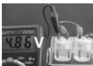
Figure 5 Using wells 1 + 2 as Galvanic Cells red: \text{Cl}_2(\text{g}) + 2\text{e}^- \rightarrow 2\text{Cl}^-(\text{aq}) + 2\text{H}_2\text{O} Ox: \text{H}_2(\text{g}) + 2\text{OH}^-(\text{aq}) \rightarrow 2\text{H}_2\text{O} + 2\text{e}^-
