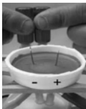
Figure 17 Bottle Hofmann 1: \text{Na}_2\text{SO}_4(\text{aq}) + red cabbage juice
