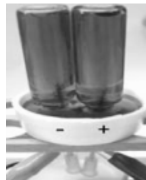
Figure 18 Bottle Hofmann 2: red: 2 \text{H}_2\text{O} + 2 \text{e}^- \rightarrow \text{H}_2(\text{g}) + 2 \text{OH}^-(\text{aq}) ox: \text{H}_2\text{O} \rightarrow \frac{1}{2} \text{O}_2(\text{g}) + 2 \text{e}^- + 2 \text{H}^+(\text{aq})
