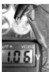
Figure 10 Potential between Zinc/copper half cells in one well of Wellplate 6.
